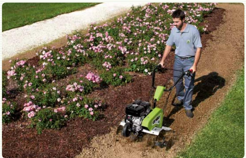
**The side discs** are necessary to balance the machine and to mark out the tilled area. When working on softer soil, the side discs are recommended to prevent the tilled soil from covering the new plants and damaging their roots.
