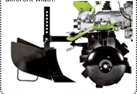
The standard **tiller** is 99 cm wide. The tines shaft is **hexagonal** and the **enlarged** tines are made of hardened steel and fixed via bolts.
