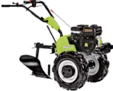
The **front transfer wheel** is equipped with a spring device that blocks it automatically into the working position or into the transfer position.
