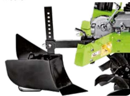
The standard **tiller** is 99 cm wide. The tines shaft is **hexagonal** and the **enlarged tines** are made of hardened steel and fixed via bolts. The tiller width can be increased to 72 or 125 cm fitting the extensions.
