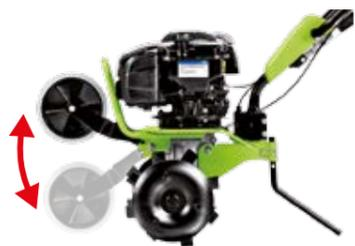
The G Z1 and G Z2 have a standard **tiller** composed of 4 banks of tines 57 cm wide with side discs. Its possible to increase the width up to 80 cm or to shorten it to 35 cm (2 banks). The G Z3 is delivered as standard with an extension kit giving 6 banks of tines. Maximum tilling depth is 28 cm. All tines are manufactured from special tempered steel and are held securely in place with bolts.
