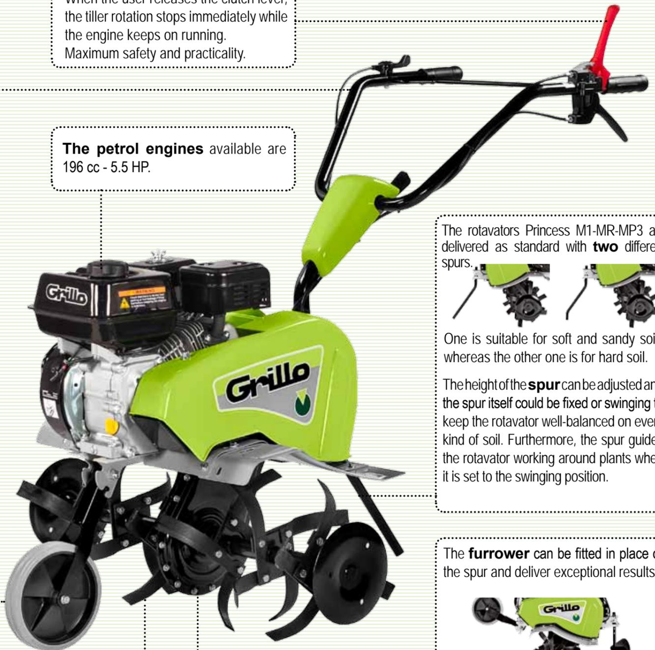
The rotavators Princess M1-MR-MP3 are delivered as standard with **two** different spurs.
