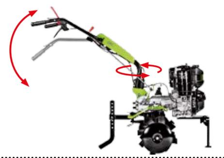
The machine is equipped with **2 PTOs**: the upper one runs at the engine rpm in anti-clockwise rotation and has a 11UNI 221 splined shaft; the lower one is synchronised with gearbox speed in clockwise rotation and has a 13 UNI 221 splined shaft.
