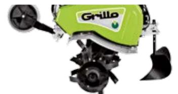
The **tiller** has a width of 83 cm and can till the ground up to 32 cm depth. It is composed of six tine-holders plus side discs and is tightly fixed to the tiller axle via M10 bolts. The tines are made of tempered steel.
