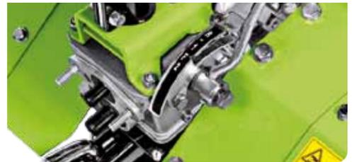
The **spur** is swinging and height-adjustable in 8 positions. **The adjustable furrower** is attached once the spur has been removed and allow to carry out furrows of different widths.
